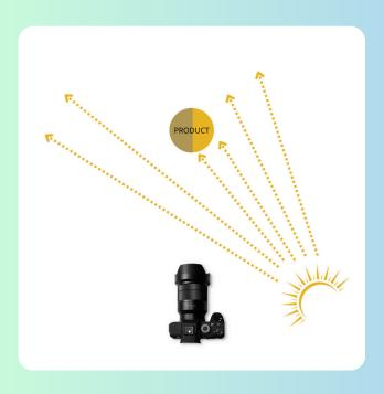
Natural light illuminates the right part of the frame, shining on the product at a 45-degree angle. As a result, the left part of the product remains underexposed (shaded).
